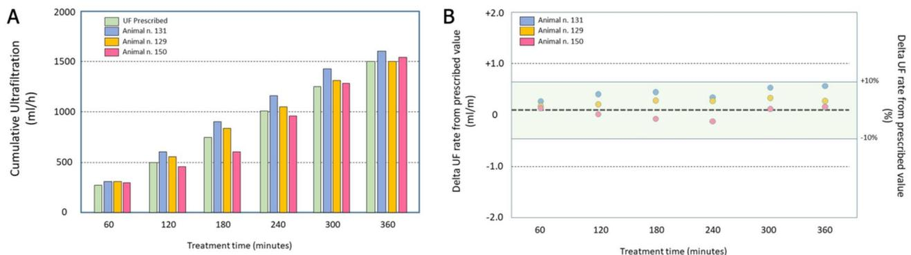
**Fig. 8** **A** Cumulative ultrafiltration volume. **B** Percentual variation between prescribed versus delivered ultrafiltration rate. Reproduced with permission from Karger. UF indicates ultrafiltration
